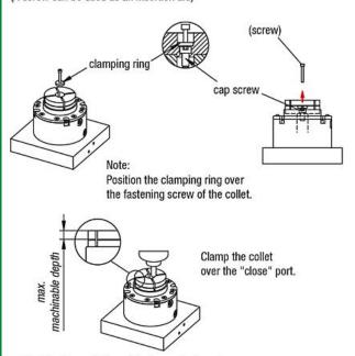
Machine the collet to suit to the workpiece shape.
