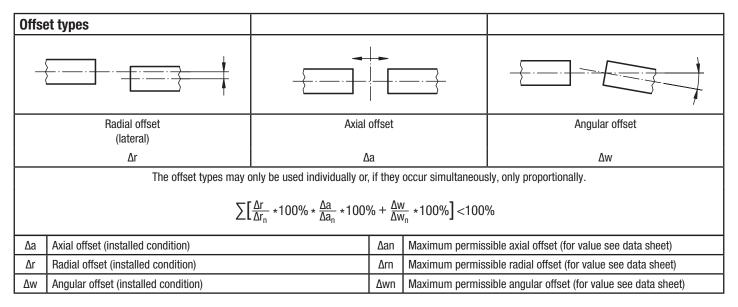
With rigid couplings, compensation of misalignments is not possible. They should therefore only be used with precisely aligned shafts. Shocks and vibrations are transmitted undamped.
