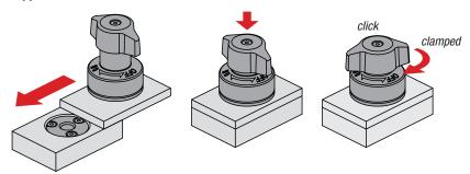
Ensure that the twist knob is in the "OFF" position.
