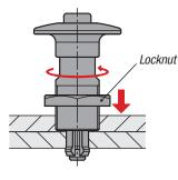
Screw the locking pin in the reverse direction till both plates come together, then secure with the locknut.
