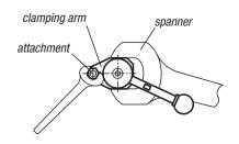
When mounting an attachment on the clamping arm, use a spanner to lock the arm and prevent it from turning.
