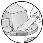
Repairs using epoxy liquid metal
