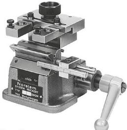
Size 0 Form B with V-block and bush holders, adjustment range of holders: 64 mm
